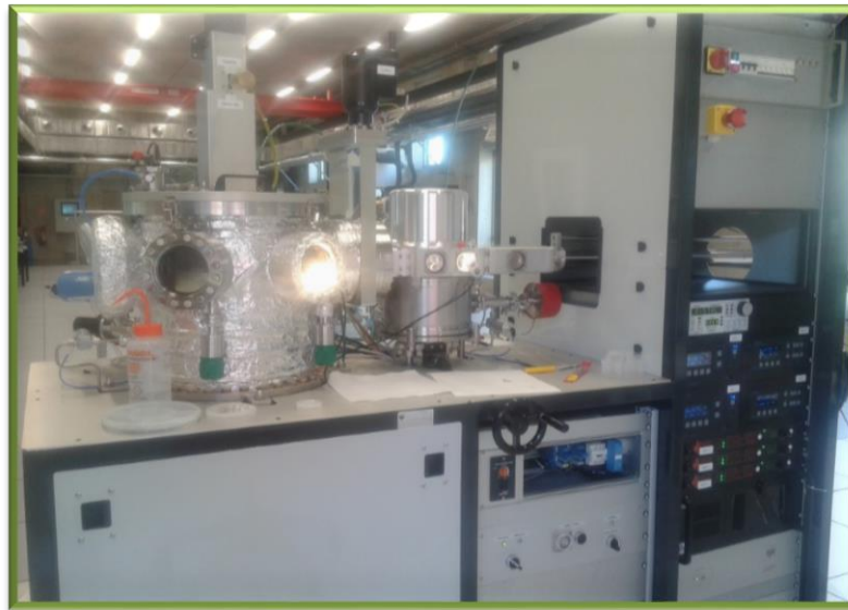
FIGURE III.2: The Physical Vapor Deposition – IJL Nancy.
