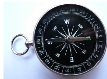
FIGURE 1.1: Dry magnetic compass.
