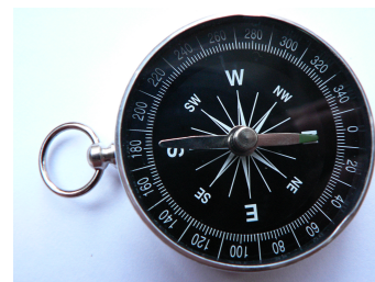
FIGURE 1.1: Dry magnetic compass.
