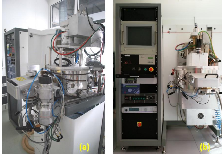
Figure 4.2: Experimental setups used for the deposition of (a) Aluminium (AC450); (b) ZnO (DP650).
