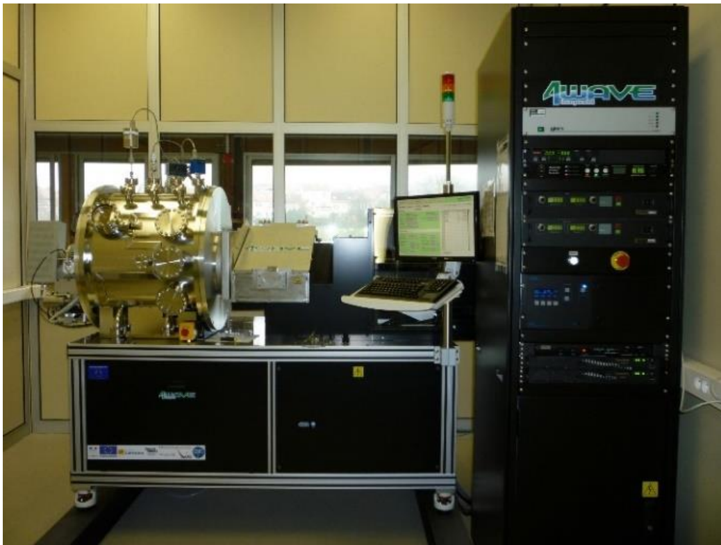
Figure 3.7: Experimental setup used for the UV lithography (SUSS MJB4) (Top) and Ion Beam Etching (4Wave) (Bottom).
