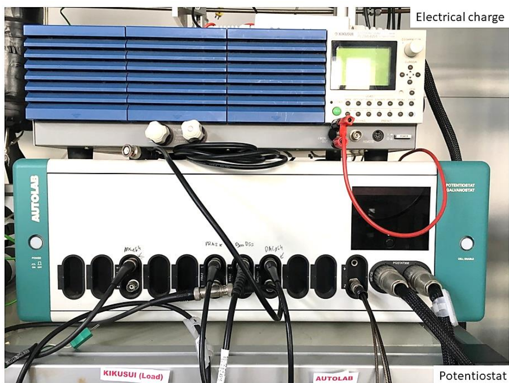
Figure 2.10 The Autolab Potentiostat at the bottom, and KIKUSUI (charge) on the top
