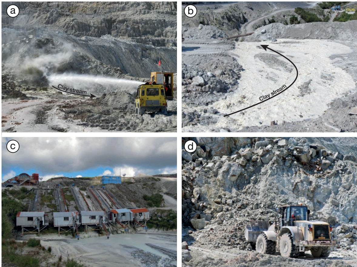
Figure 1.9: Imerys kaolin extraction methods at St Austell. Hydraulic mining use high pressure water to blast the kaolin out of the clay matrix (a). The resulting “clay stream” flows down into the pit sink (b) and is then pumped to the in-pit processing loop (c). (d) Cut and carry operation.
