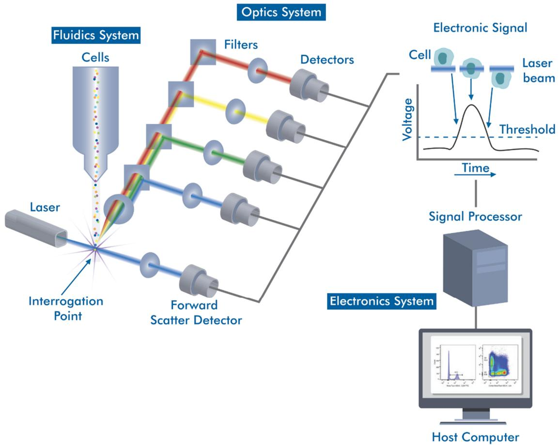
**Figure 30: Basic components of a flow cytometer.**
