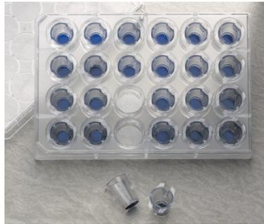
**Figure 29: Photography of Fluoroblok inserts to use with 24-well companion plate.**
