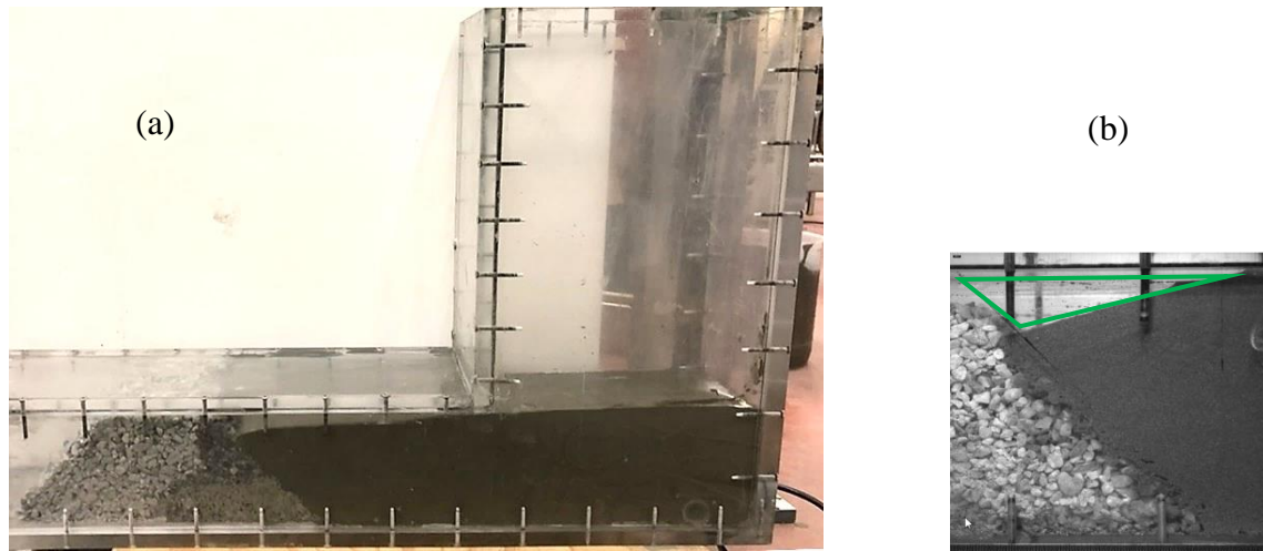
Figure 5-11: a) Tilt of the backfill slurry surface ( C_w=70\% ) during filling, b) Unfilled portion at the top of the barricade after the drainage and sedimentation process; sand ( 0/400\mu\text{m} ) was used instead of the tailings (see Nujaim et al., 2018).
