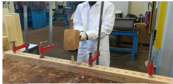
a) Assembly of beams
