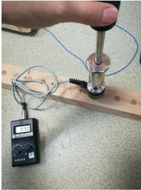
Figure 2.21: Measurement of moisture content of a beam using the H-DI 3.10K moisture meter
