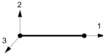
Figure 3.30: Local axes for beam element
