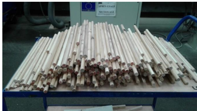
Figure 2.3: Typical produced compressed spruce dowels
