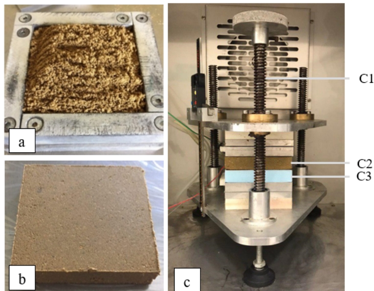
Figure 2.5: a) mold of sample preparation for centred hot plate tests b) compacted soil sample for centred hot plate test c) test assembly C1) Manually Compressing screw (Tightening device) C2) soil sample C3) reference material.
