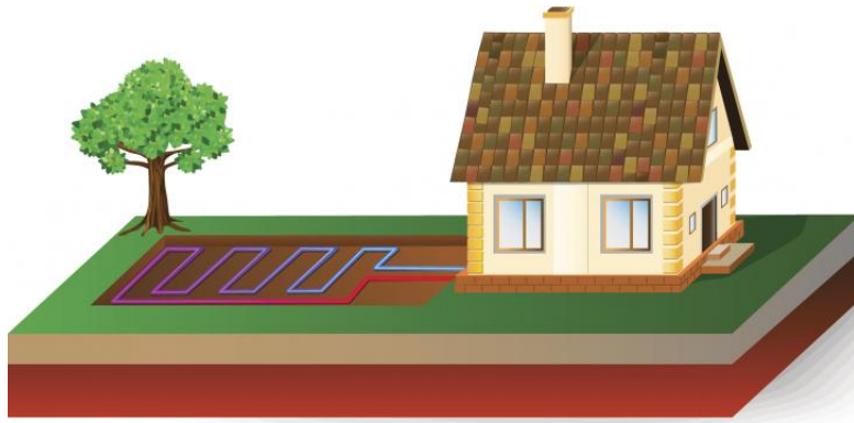
Figure 1.3: Thermal energy storage using horizontal heat exchanger loops (www.greenliving.lovetoknow.com).
