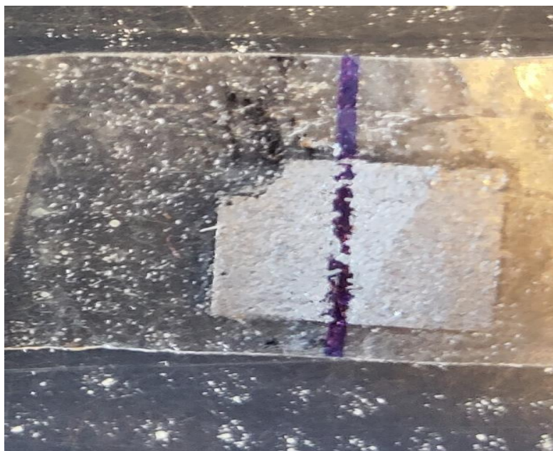
Figure 2. Preliminary result of the patterning process of graphite on the scotch tape.
