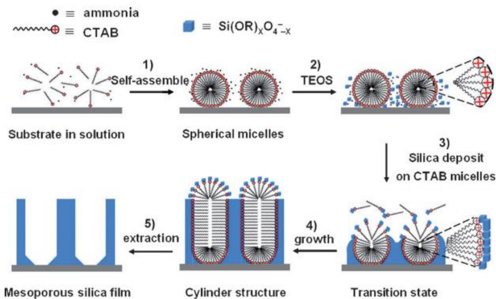
Figure 9 - Formation process of ordered mesoporous silica films with perpendicular mesochannels by the Stöber-solution spontaneous growth procedure [97]
