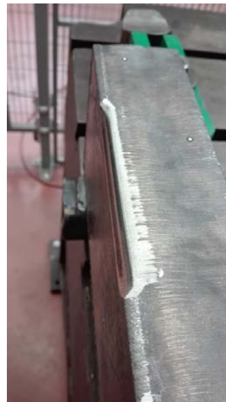
FIGURE 4.15: Essai MA : Arrondi meulé
