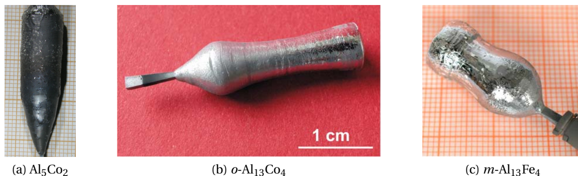
Figure 1.22: (a) \text{Al}_5\text{Co}_2 single crystal grown from an Al-rich solution of initial composition \text{Al}_{76}\text{Co}_{24} [13, 106], (b) o\text{-Al}_{13}\text{Co}_4 single crystal grown from an Al-rich solution of initial composition \text{Al}_{86.5}\text{Co}_{13.5} and (c) m\text{-Al}_{13}\text{Fe}_4 single crystal grown from an Al-rich solution of initial composition \text{Al}_{89.5}\text{Fe}_{10.5} [103].
