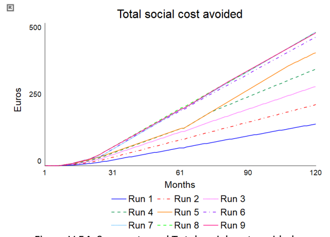
Figure V.54. Scrap rate and Total social cost avoided Run 1: 0.2, Run 2: 0.3, Run 3: 0.4, Run 4:0.5, Run 5:0.6, Run 6: 0.7, Run 7: 0.8, Run 8: 0.9, Run 9: 1
