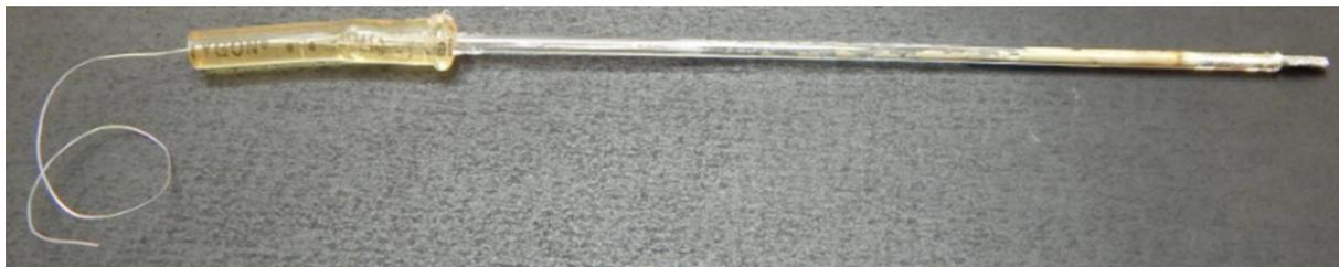
Figure 3.4: Platinum mesh based counter electrode.
