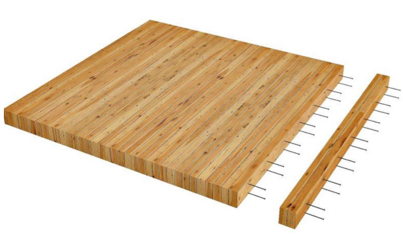
Figure 2.30 : Panneau en bois lamellé-cloué (Nailed laminated timber)
