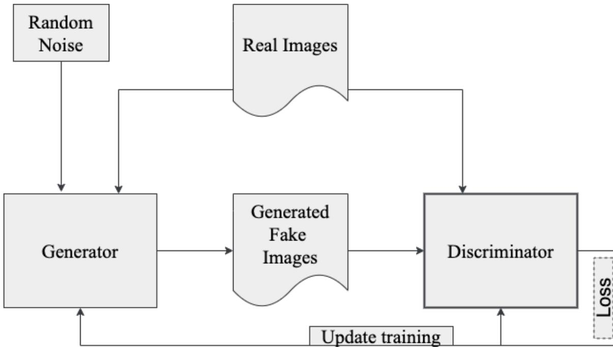
FIGURE 2.13 – Schematic diagram of GAN for computer vision
