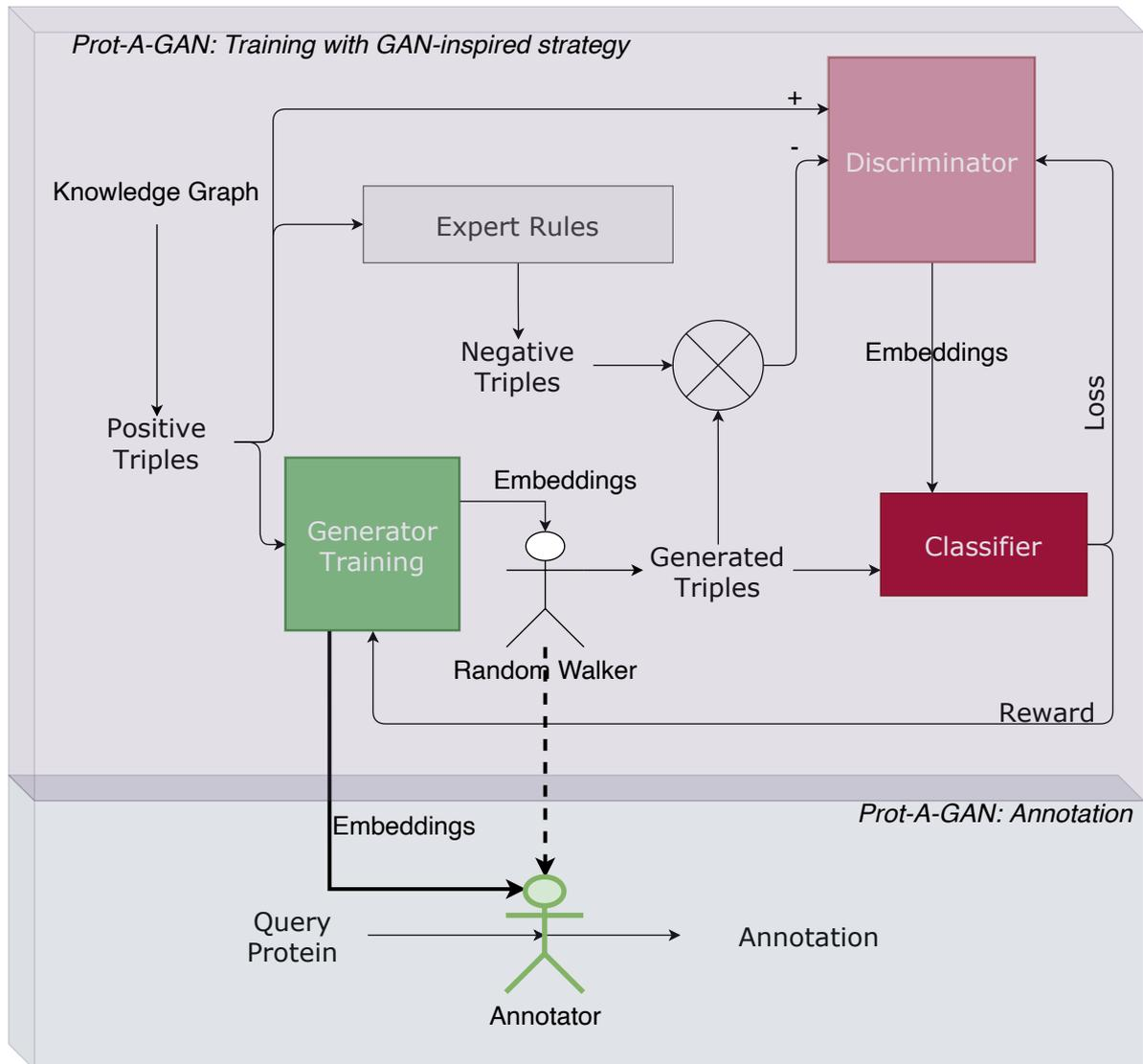
FIGURE 6.2 – Schematic diagram of the proposed Prot-A-GAN framework (Annotation). Once the model is trained following the Figure 6.1, the Generator parameters i.e.  $\Theta_G^V$  and  $\Theta_G^R$  are used to guide the random-walker (now annotator) to perform the annotation task. It takes a protein ID as input, the annotator moves around the knowledge graph to find relevant GO terms using the relevancy score computed from  $\Theta_G^V$  and  $\Theta_G^R$ .
