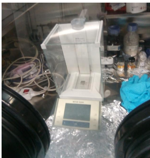
Figure II-15 : Semi-microbalance Mettler Toledo.
