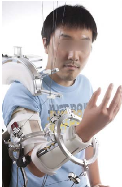
Figure 2.10: Carex:wearable exoskeleton [MA12]
