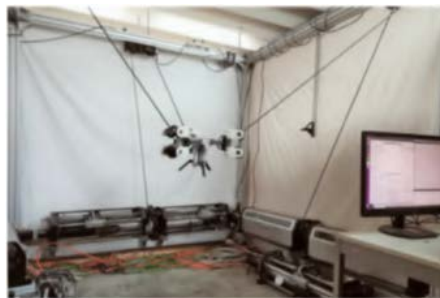
Figure 2.21: CDPR prototype developed by Eda et al. [IBC19]
