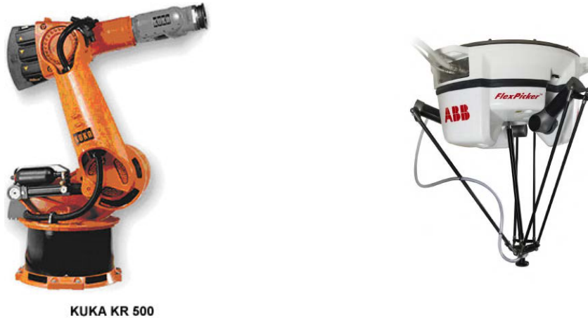
(a) A serial manipulator from KUKA robotics [Kuk] (b) A parallel manipulator from ABB [Abb]
