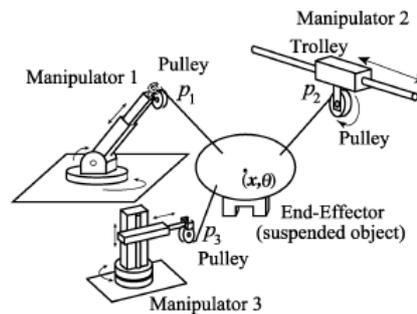
Figure 2.13: Under-constrained CDPR used for study by [YYM02]
