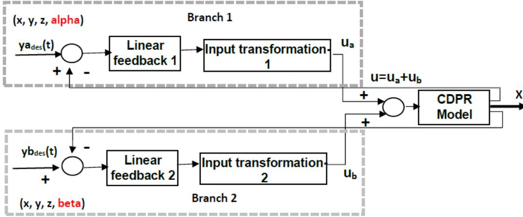
Figure 4.16: Block diagram of the Modified Feedback Linearization
