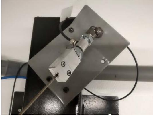
Figure 5.3: K100, a tension force sensor from SCAIME and the anchor plate for attaching the cable
