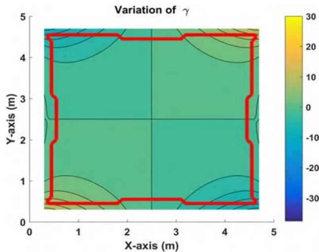
Figure 3.8: Orientation angle ( $\gamma$ ) at  $z = 1.5$  m
