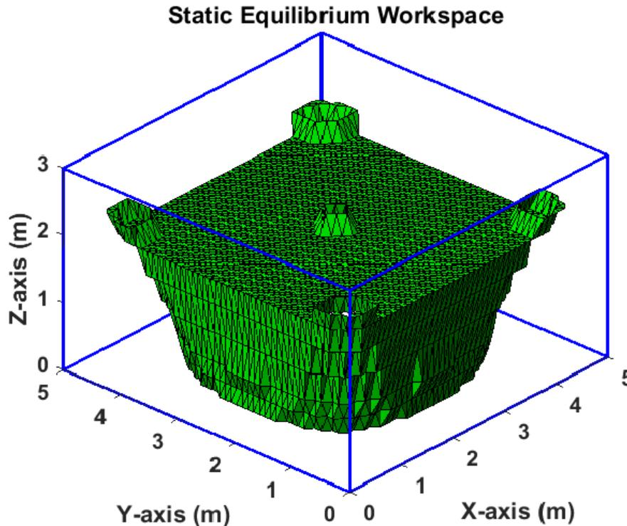
Figure 3.3: SEW of the cable driven robot
