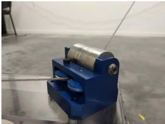
Figure 5.4: Cable guide for the CDPR
