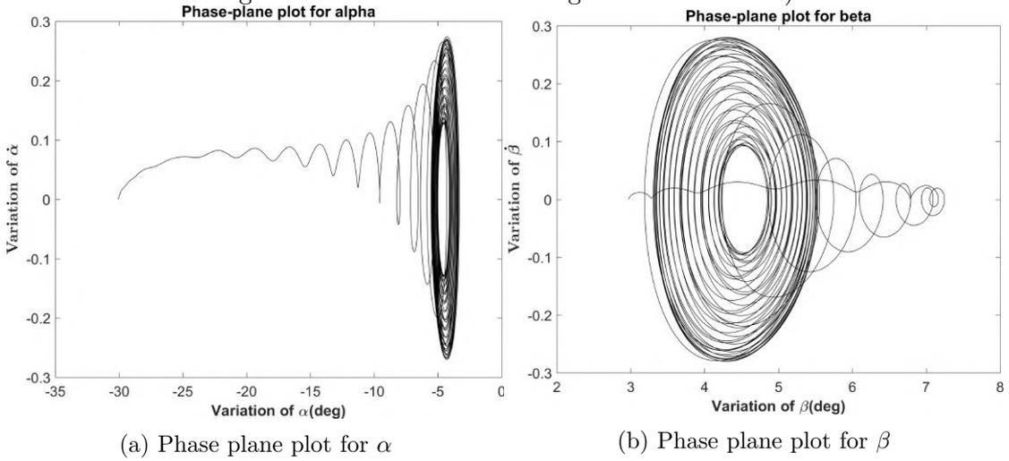
Figure 4.10: Phase plane plot for the uncontrolled dof
