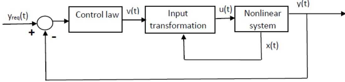
Figure 4.1: Block diagram for IOFL
