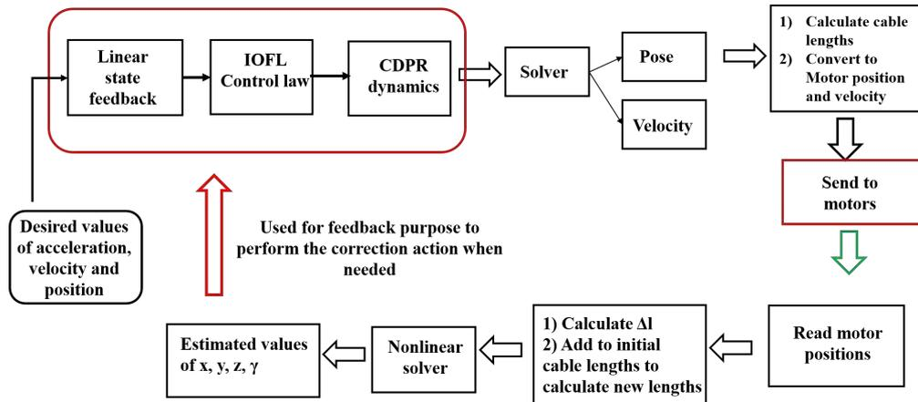
Figure 5.7: Block diagram for control approach
