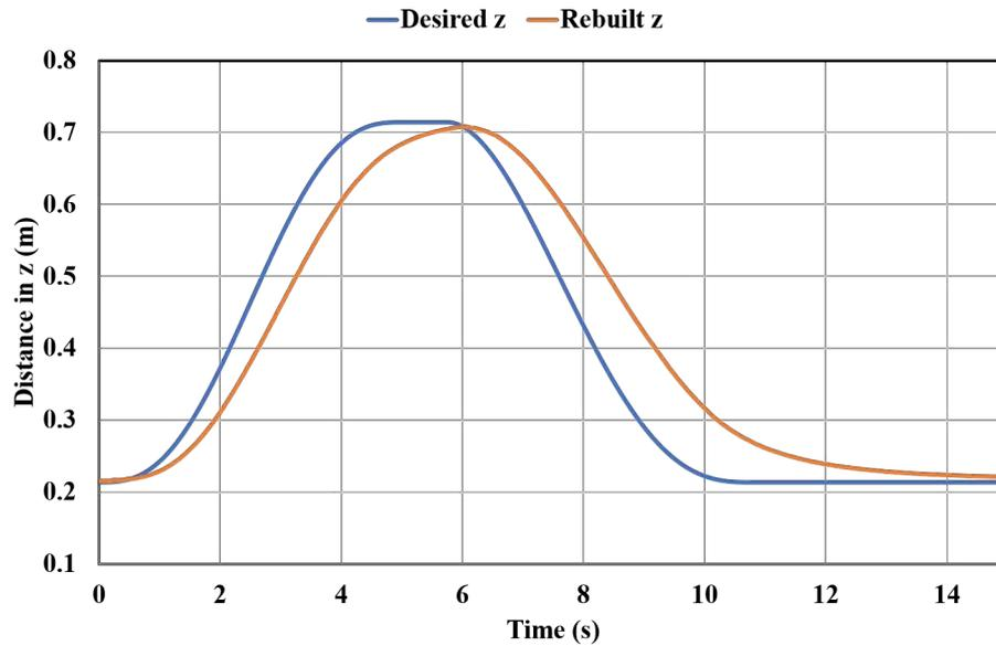
Figure 5.17: Comparison between the desired value of  $z$  and the rebuilt value of  $z$  from the motor position for a desired velocity of  $0.1\text{ m/s}$  for the up and down movement of the MP
