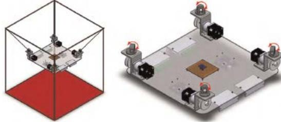
Figure 2.19: Underactuated CDPR prototype used by [LL16a]
