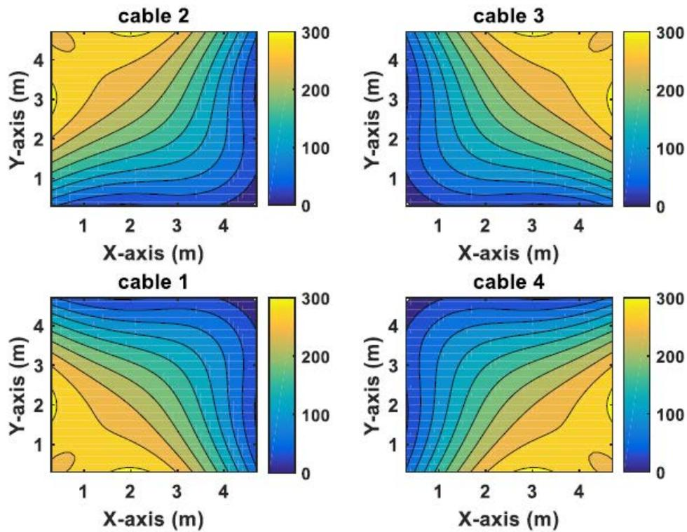
Figure 3.5: Cable tensions at  $z = 1.5$  m
