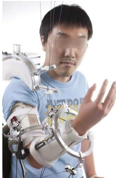
Figure 2.10: Carex:wearable exoskeleton [MA12]
