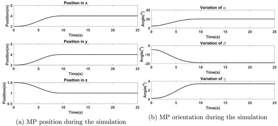
Figure 4.7: MP behavior during simulation case (b)
