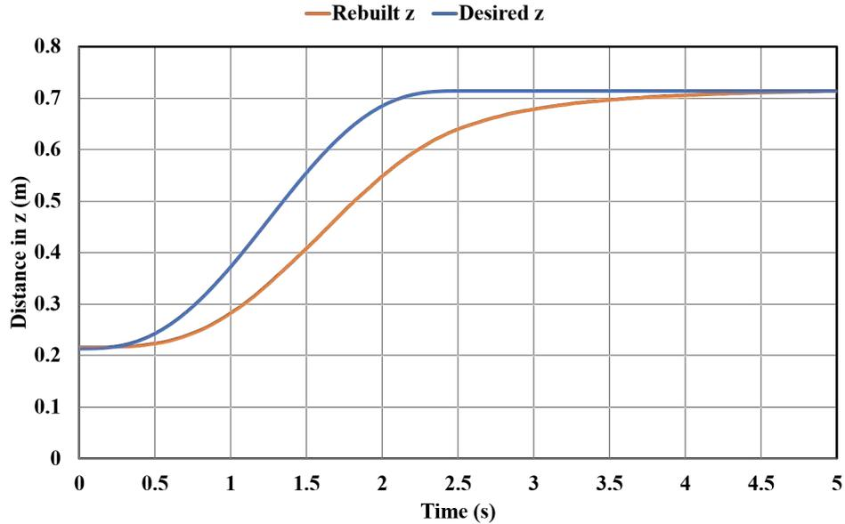
Figure 5.13: Comparison between the desired value of  $z$  and the rebuilt value of  $z$  from the motor position for a desired velocity of  $0.2 \text{ m/s}$  for the MP
