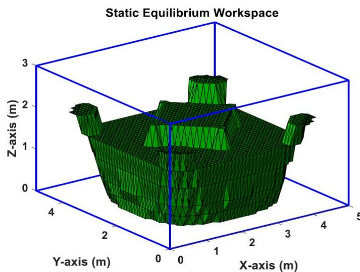
Figure 3.12: SEW for a payload of 40 kg on the MP
