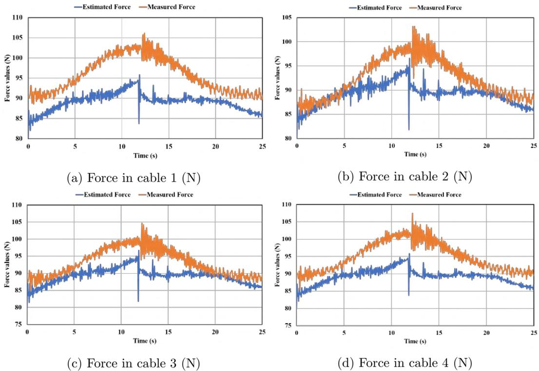
Figure 5.16: Comparison of the estimated and measured cable forces for moving the CDPR from home position to a distance of  $0.5 \text{ m}$  and returning back to the home position with a desired velocity of  $0.05 \text{ m/s}$ .
