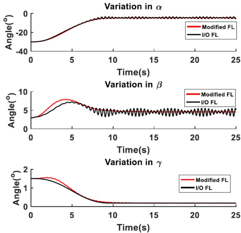
Figure 4.20: Platform orientation angle ( $\alpha$  and  $\beta$ )
