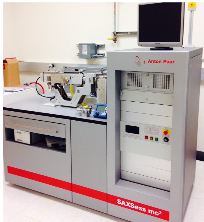
FIGURE 2.8: The picture of the GiSAXS instrument used
