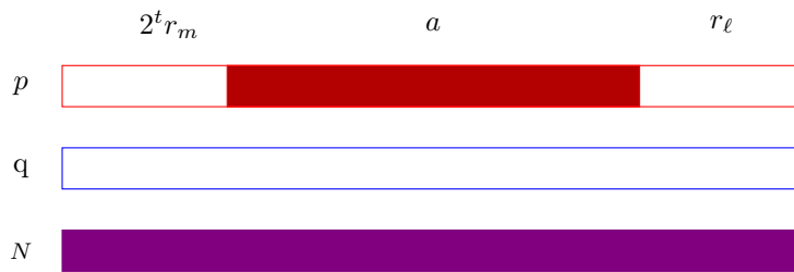
Figure 6.4: Factorization of N = pq given contiguous known bits of p in the middle.
