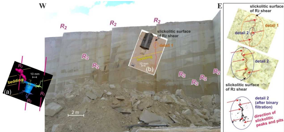
Figure 13. Correlation of results obtained with help of the CT 3D model in (a) the W–E direction and (b) microstructural analysis of a high-resolution photo of the vertical section of the studied sample for experiment #7 with outcrop scale structural patterns in the quarry excavating the Lavoux limestones. Note, the elements of the roughness for the slickolitic surface of R 2 shears affected the dissolution pathways and geometric shape of the principal wormhole, shown in pink in the inset in (a).
