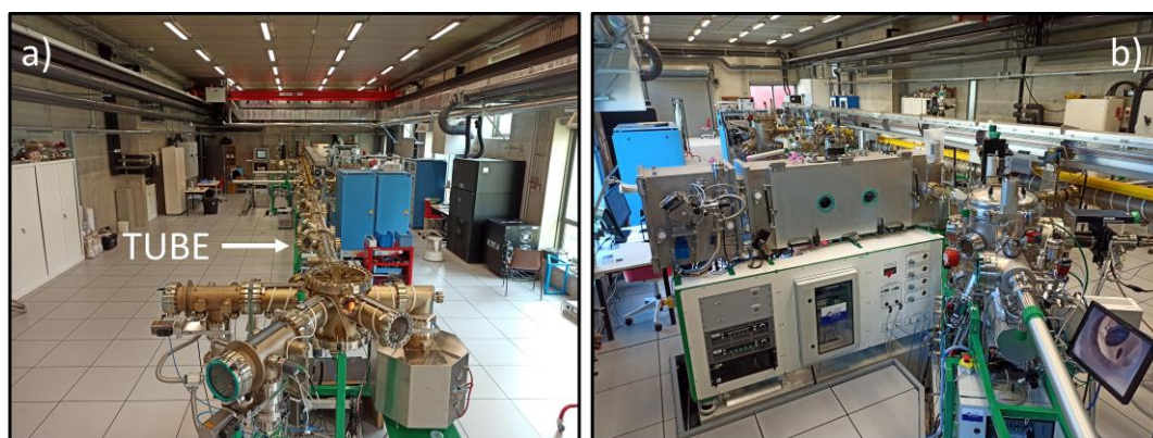
Figure 2.4 a) Transfer Technology Office (TTO) part of the TUBE. b) Semi-industrial and standard sputtering machine connected to the TUBE.
