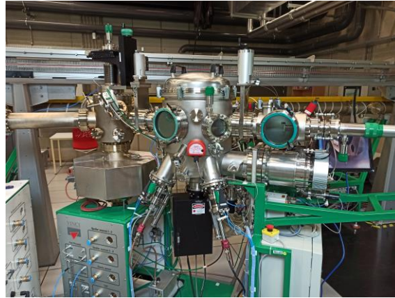
Figure 2.6 Standard sputtering chamber connected to the TUBE.
