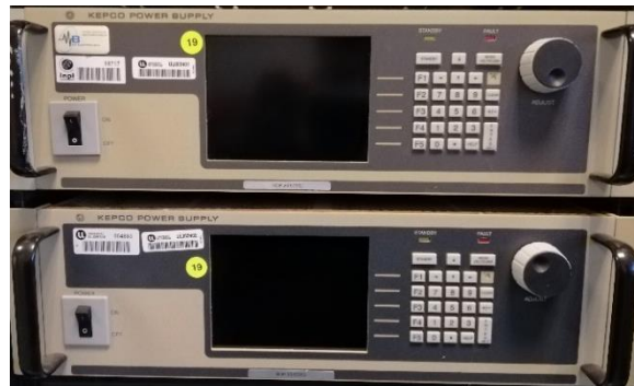
Figure A- 4 Kepco Power Supply.
