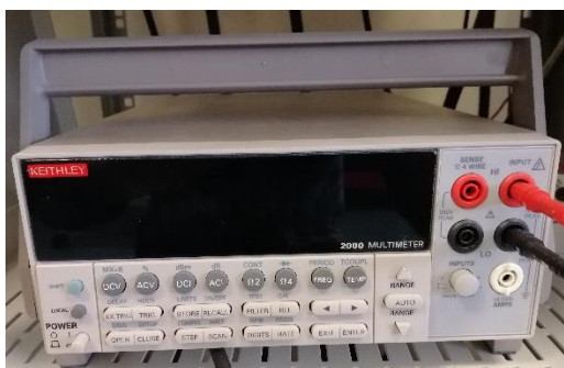
Figure A- 2 Nano-voltmeter: Model 2000 multimeter.
