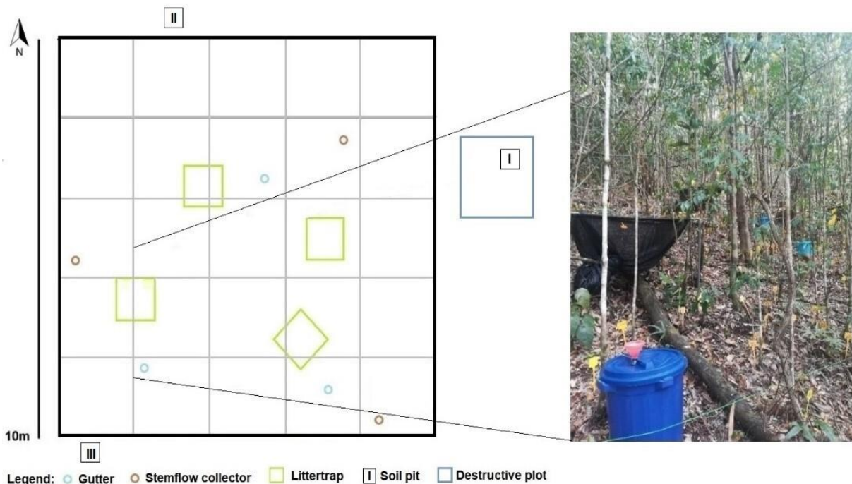
Figure 9 Overview of the biogeochemical plot and the monitoring instruments (gutter, litter trap and stemflow collector) in an ultramafic ecosystem dominated by the Ni hyperaccumulator Phyllanthus rufuschaneyi in Sabah, Malaysia
