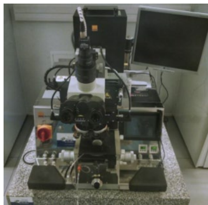
Figure 2-3 UV lithography machine (MA6, SUSS, Germany).
