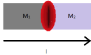
Figure 1.1: Schematic representation of Peltier experiment
