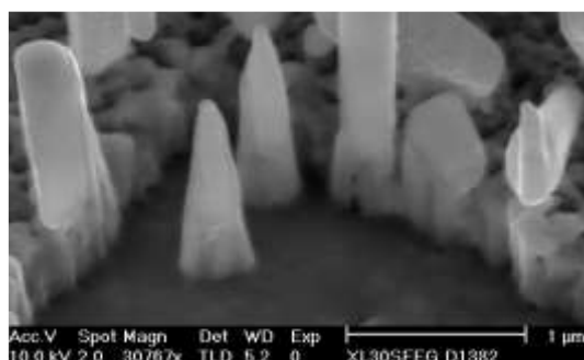
Figure 5.3: SEM image of Sn nanowires [255]
