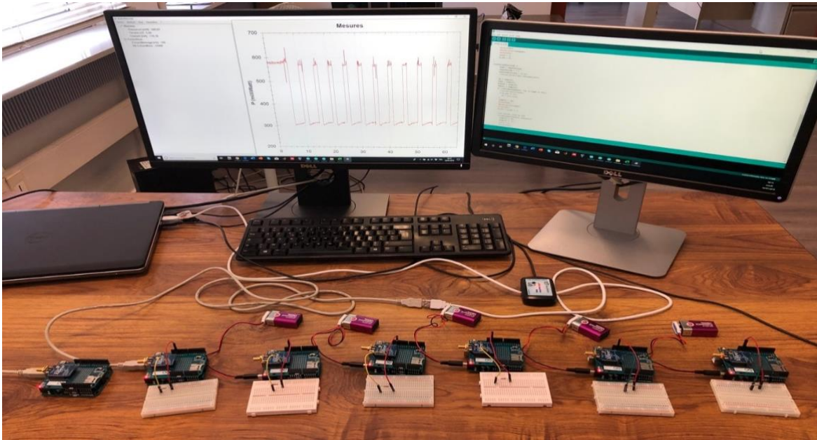
Figure 82 Six-node chain testbed
