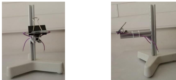
Figure 4.4 (P(VDF-TrFE) film holder view (a) Front view (b) Side view
