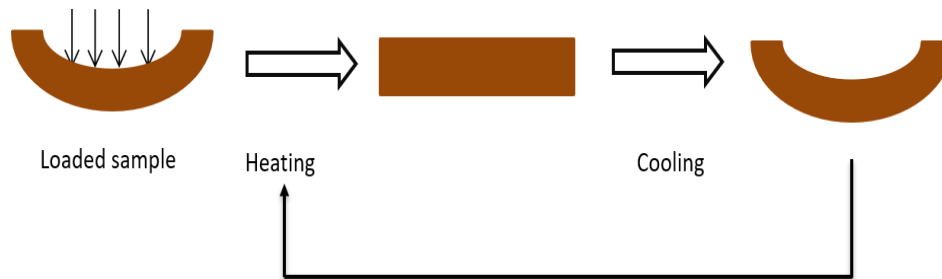
Figure 3.6. Schematic representation of the simulation of the two-way shape memory effect.
