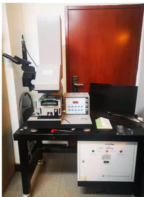
Figure 2.9 UV lithography machine.
