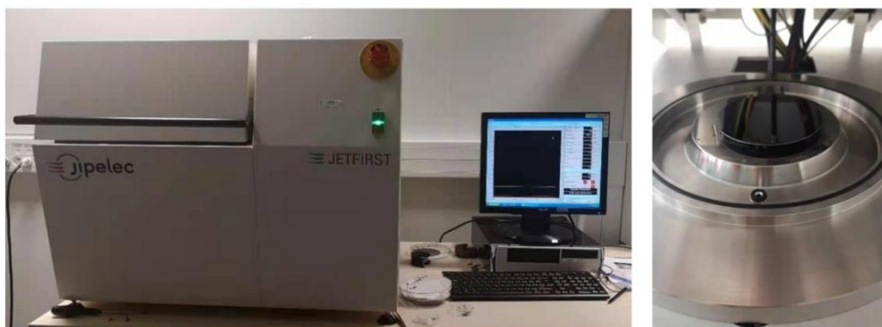
Figure 3. 2 Rapid thermal annealing equipment (RTA).
