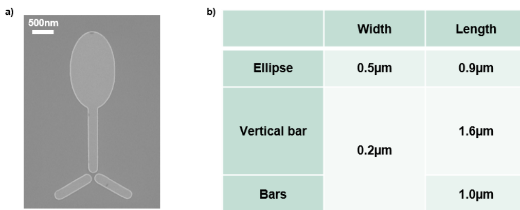
Fig.4-10: a) SEM image of 1-stage disconnected structure with 20 nm-thick Permalloy; b) dimensions of the elements. The half diameters are given for the nucleation pad. The vertical bar length is taken from the edge of the pad to the end of the element.
