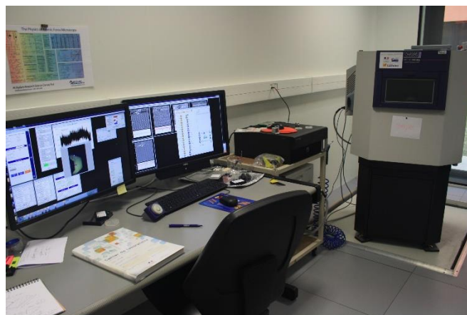
Fig.2-14: MFM set up used for this work.
