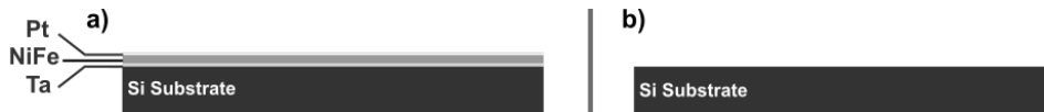
Fig.2-1: a) Ta(3nm)/NiFe(20nm)/Pt(3nm) deposited with magnetron sputtering on top of Si substrate for the etching process and b) plain Si substrate for the lift-off process.
