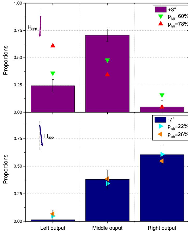
Fig.4-26: Observed activated outputs with a)  $+3^\circ$  tilt, results over 50 structures observed 6 times yielding 300 experiments considered independent and b)  $-7^\circ$  tilt, results over 12 structures observed 11 times yielding 132 experiments considered independent. Proportions of avalanches 68% and 54% for the  $+3^\circ$  and  $-7^\circ$  tilts respectively.
