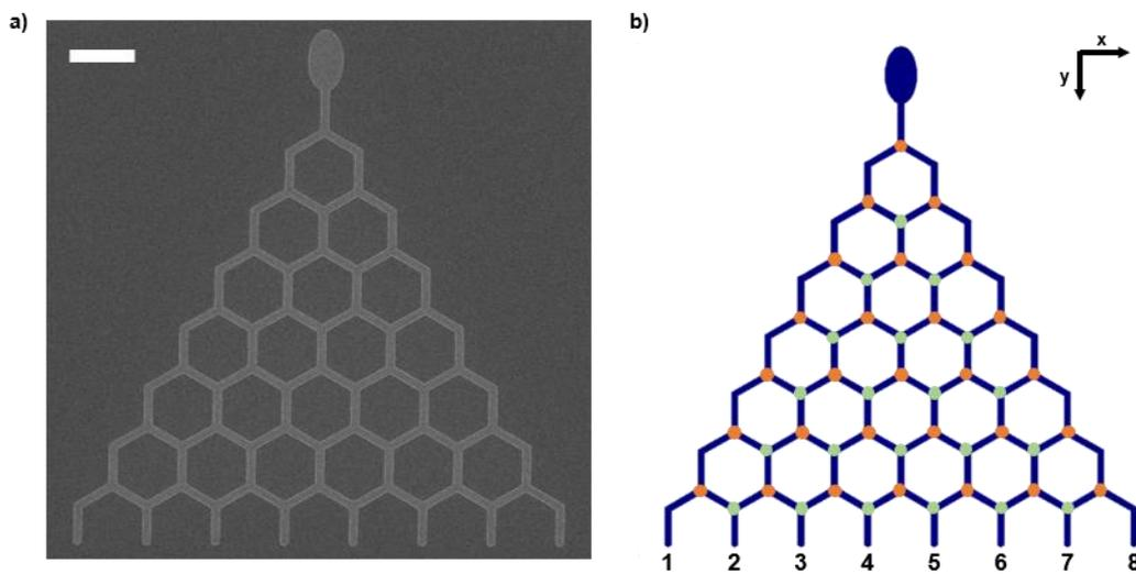
Fig.4-27: a) SEM image of the 7-stage structure, elements are 200 nm wide, elements are 1.2  $\mu\text{m}$ -long, upper element connected to the pad is 1.3  $\mu\text{m}$ -long; b) identification of the intersection (orange disks), pinning points (green disks) and the outputs of the structure (indexed from 1 to 8). Scale bar is 2 $\mu\text{m}$ .
