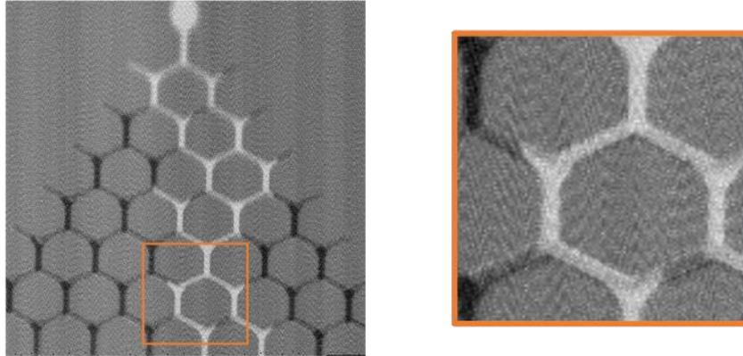
*Fig.4-48: Observation of reversals using STXM of a propagation on another structure and close-up view of the framed part. White contrasts correspond to the reversed elements of the structure. Experiments performed by Dr. K. Ait Oukaci, Prof. F. Montaigne, Dr. R. Belkou and me.*
