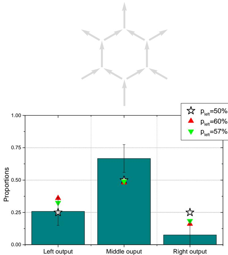
Fig.4-25: Observed activated outputs. Results are summarised over 21 structures (with a field alignment of  $\pm 0.5^\circ$ ) yielding 87 experiments considered independent, 76% of them form avalanche-like reversals and represented here.
