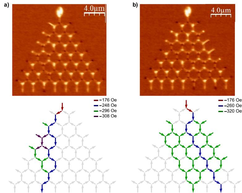
Fig.4-38: Examples of experiments with chain-like reversals and the reversals after the output is reached: a) output 2 is activated after a 2-step avalanche at  $-176$  Oe and  $-248$  Oe, then at  $-296$  Oe green spins reverse starting from pinning point (6, 3) along with outer second left diagonal element and at  $-308$  Oe, purple spins reverse from pinning points (4, 1 and 2) up to both upper elements of pinning point (3, 1).
