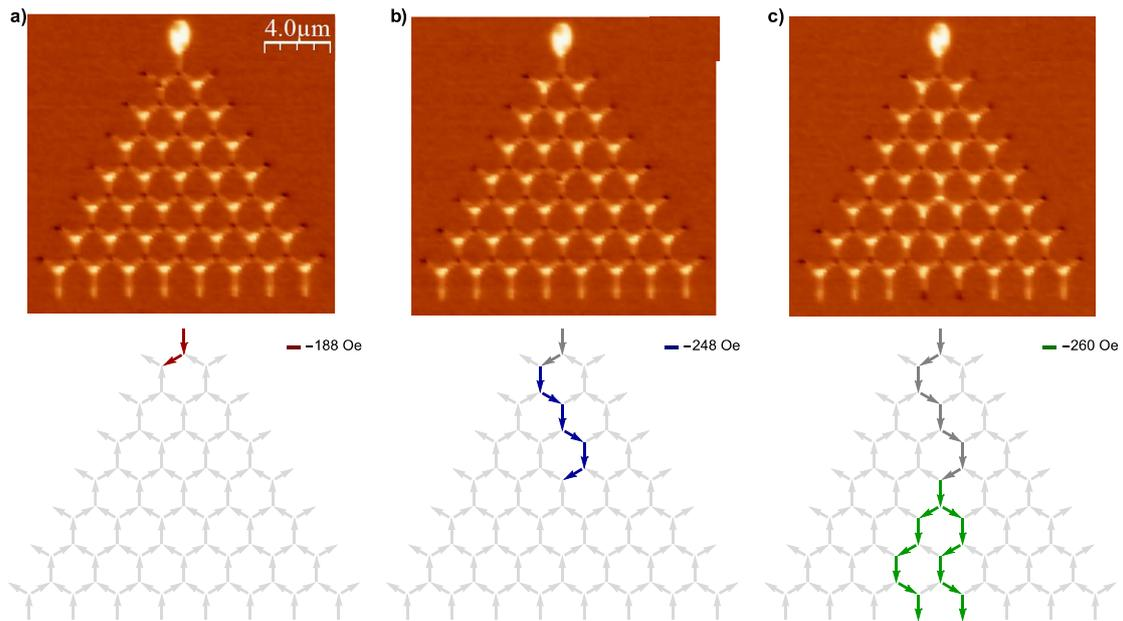
Fig.4-39: Experiment with a domain propagation in three events: a) at  $-188$  Oe, injection and propagation of the nucleated domain wall up to pinning point (1, 1); b) at  $-248$  Oe, depinning and propagation of the domain wall up to pinning point (4, 3); c) at  $-260$  Oe, depinning and propagation with intersection (5, 3) being a splitting point. Spins in darker grey have reversed at lower fields.
