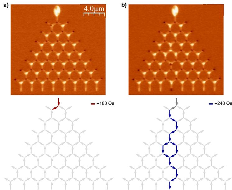
Fig.4-40: Example of ambiguous path to reach the end of the structure: a) at  $-188$  Oe, injection and domain wall propagation from the pad to pinning point (1, 1); b) at  $-248$  Oe, depinning and chain-like reversals up to intersection (4, 2) at which both diagonal elements have reversed, following reversals join at pinning point (5, 3) then activate output 4. Spins in darker grey have reversed at lower field.
