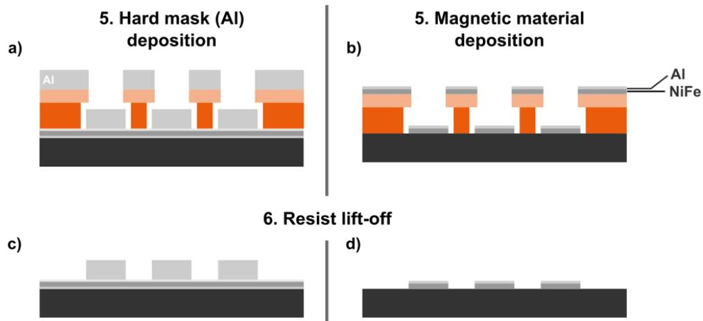
Fig.2-3: a) Deposition by *e*-beam evaporation of 100 nm-thick Al layer acting as hard mask in order to perform IBE and b) NiFe(20)/Al(3) also by evaporation for the lift-off process; c)-d) result of lift-off of the remaining resist and surplus of material by Remover1165 hot bath and sonication.
