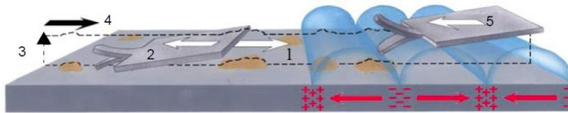
Fig.2-13: From the Veeco Dimension 3100 Manual: 1<sup>st</sup> and 2<sup>nd</sup> step, the probe traces and retraces the surface to get the topography in tapping mode; 3<sup>rd</sup> step: the probe ascends in the Lift Scan Height or Nap Height; 4<sup>th</sup> and 5<sup>th</sup> steps: probe traces and retraces the topography.
