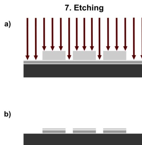
Fig.2-4: a) Etching step and b) final sample of the etching process.
