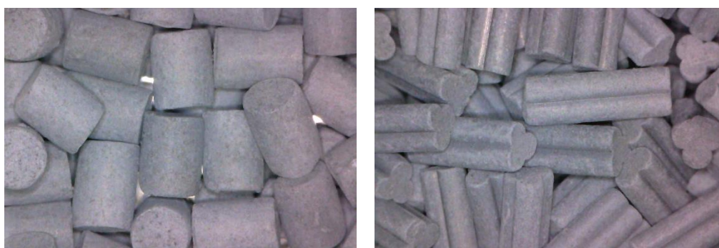
Figure 3 Cylindrical pellets and trilobes of SiC.
