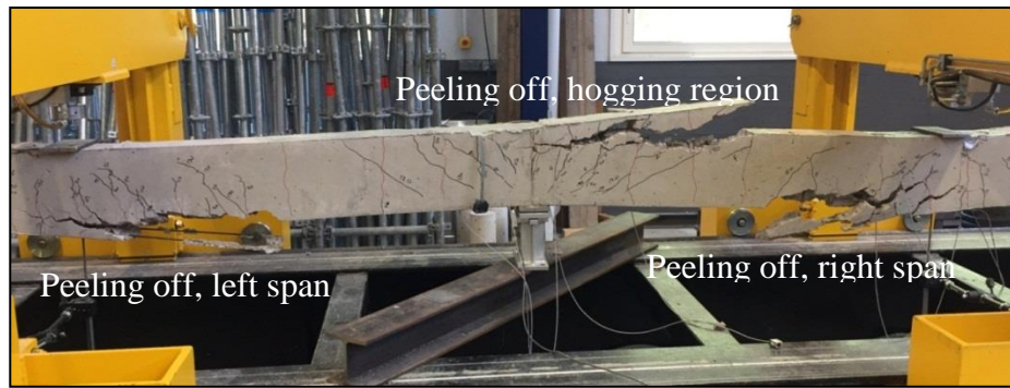
Figure 2-13 : Failure mode of beam BC3-L
