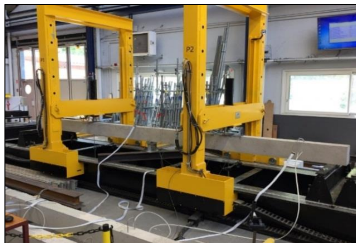
Figure 3-3 : Test setup and the instrumentations used for testing beams.
