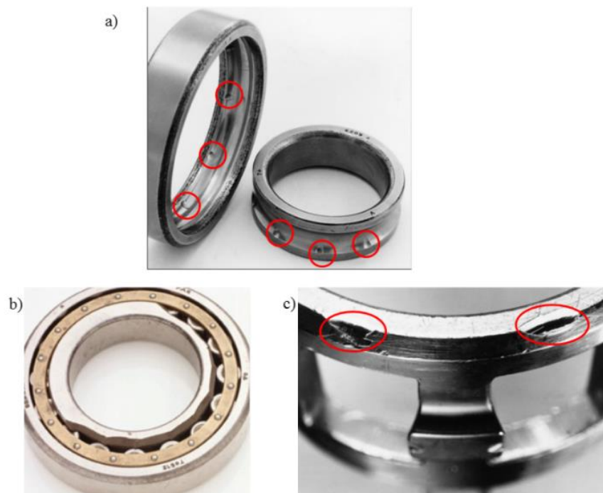
Figure 2.5 Damages of bearings due to disassembly operations: (a)-Brinell marks appear as indentations in the raceways, increasing bearing vibration, (b)-supporting lip is partly or completely broken off or crack and (c)-metal cage with dents (Ag & Kg, 2004)
