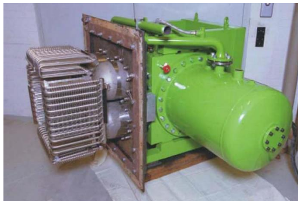
Figure 1.5: The 35-kW Stirling engine developed in 1996 [18]
