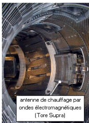
FIGURE 1.9: Antenne de chauffage.
