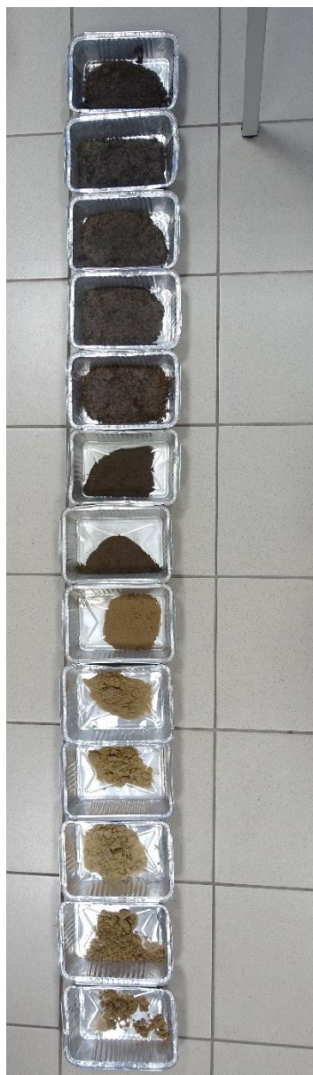
Fig. III.S 5.5 Example of soil color evolution with depth for Block 2, Plot 1 (pure birch) in July 2019. The top of the picture represents the topsoil (0-5 cm) and each following box the following depths (5-10, 10-15, 15-25, 25-35, 35-45, 45-55, 55-65, 65-75, 75-85, 85-100, 100-115, 115-125). We can observe here that the top horizons are the ones with the most organic matter.
