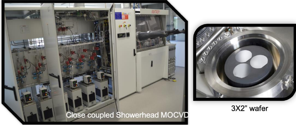
Figure 2-8: Aixtron 3x2 inch, close coupled showerhead (CCS) MOVPE system.
