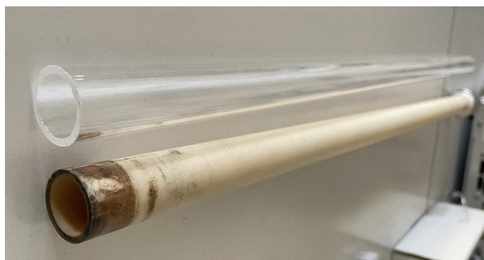
Figure 46: Fused silica and alumina flow tubes (FR2).
