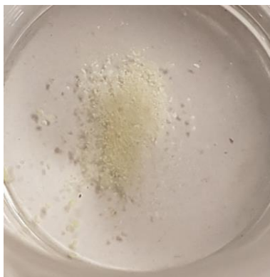
Figure 69: Solid sulfur found at the outlet of FR2.
