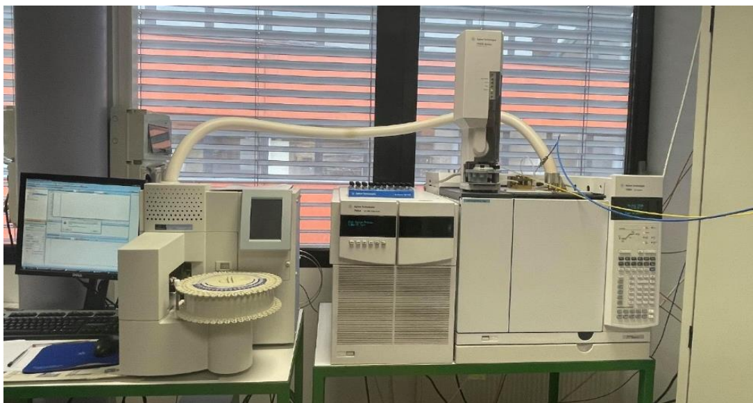
Figure 51: Picture of the GC-MS used for the analysis.
