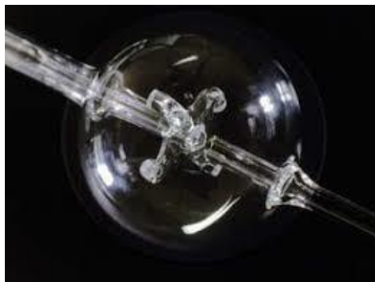
Figure 43: Picture of a jet-stirred reactor.
