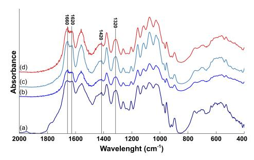
Figure 2.1. FTIR spectra of CH-17 (a), CH-19 (b), CH-20 (c) and of a commercial chitin (d).
