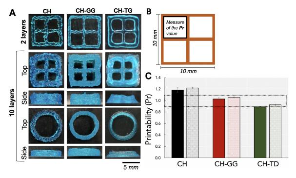
Figure 3.4. Qualitative and semi-quantitative evaluation of the printability of the three ink formulations: CH, CH-GG and CH-TG. (A) Qualitative images of 10 mm x 10 mm square and 10 mm circular constructs printed in 2 or 10 layers view form the top and from the side. (B) Representative image evidencing the pores used for the calculation of the Pr value. (C) Quantification of the printability (Pr value) of constructs made of 2 layers (full bars) or 10 layers (dotted bars) using the Pr value.
