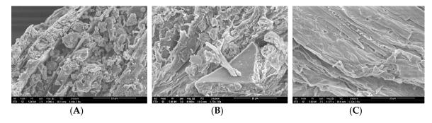
Figure 5. SEM images of (A) raw material, (B) demineralized, and (C) decolorized samples.
