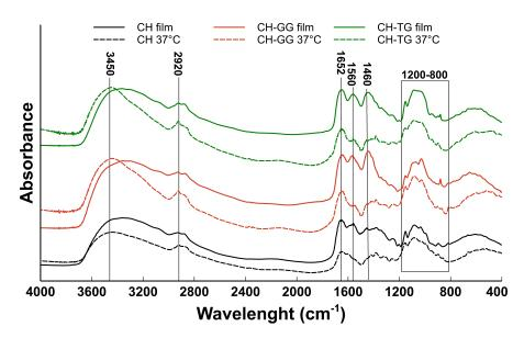
**Figure 3.2.** FTIR spectra of the ink solutions in form of film (discontinuous line) and of the lyophilized 3D printed construct after incubation overnight at 37°C for 24 hours (continuous line). Black curves correspond to the sample CH, red to CH-GG and green to CH-TG.
