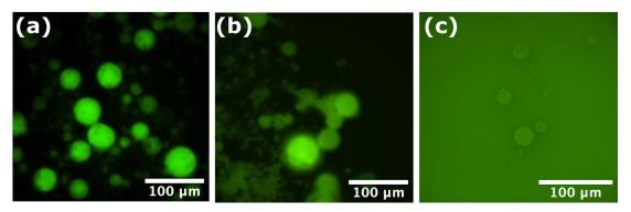
**Figure 5.8.** FITC dextran-loaded PLGA microspheres before lyophilization (a), after lyophilization (b) and after lyophilization and subsequent immersion in water for 4 hours.
