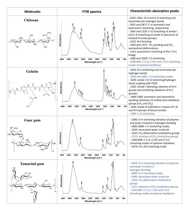
Figure B1. Summary of the FTIR spectra and characteristic absorption peaks of chitosan, gelatin, guar gum and tamarind gum. The characteristic absorption peaks for chitosan, gelatin and guar gum have been obtained from previous studies [148, 149, 150] and are reported in black. The characteristic peaks of tamarind gums were not found in the literature and are extracted from the graph and the comparison with guar gum and chitosan spectra. These and others derived peaks are reported in blue.
