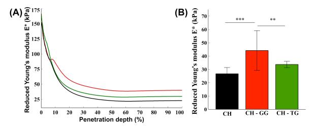
Figure 3.6. Nanoindentation of the samples CH, CH-GG and CH-TG. (A) Reduced Young's modulus vs indenter penetration depth for the samples CH (black), CH-GG (red) and CH-TG (green). (B) Average reduced Young's modulus values for the samples CH, CH-GG and CH-TG measured between 70 and 90% of penetration depth. \*\*\*p<0.001.
