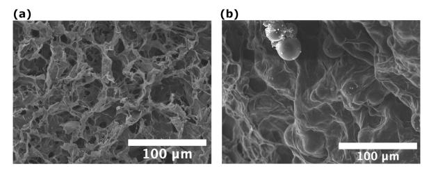
**Figure C2.** Ultrastructure (SEM) of the crosslinked microsphere-free (a) and microsphere-laden (10 mg/mL) (b) hydrogels after 7 days in PBS at 37°C.
