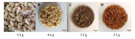
**Figure 1.** Schematic illustration of the raw material and all the other samples after the extraction steps. The weight of the raw material (**A**) after washing and drying it in the oven at 50 °C for 24 h was 5.4 g. The weight of dried demineralized (**B**), deproteinized (**C**), and decolorized samples (chitin-**D**) was 4.6, 3.2, and 2.3 g, respectively.
