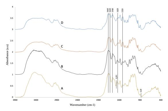
Figure 2. FTIR spectra of (A) raw material, (B) demineralized, (C) deproteinized, and (D) decolorized samples.
