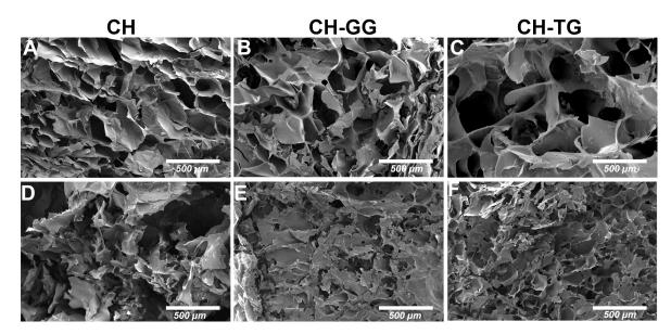
**Figure 3.7.** SEM images of the bioprinted constructs made of CH (A and D) at day 0 (A) and after 21 days in lysozyme (D), CH-GG (B and E) at day 0 (B) and after 49 days in lysozyme (E) and CH-TG (C and F) at day 0 (C) and after 49 days in lysozyme (F).
