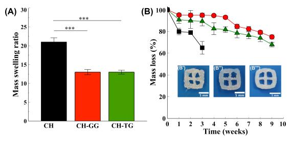
Figure 3.5. (A) Mass swelling ratio of constructs made of chitosan (CH) and tamarind (CH-TG) or guar (CH-GG) gum. \*\*\*p<0.001. (B) Degradation profile of the same constructs (Black: CH, Green: CH-TG, Red: CH-GG) and representative images of the construct CH (B') after 3 weeks in lysozyme, CH-TG (B") and CH-GG (B"') 7 weeks in lysozyme.
