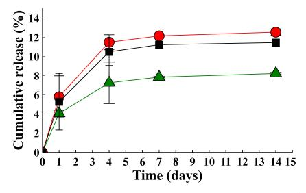
**Figure 3.8.** Cumulative release of BSA from bioprinted construct made of CH (black squares), CH-GG (red circles) and CH-TG (green triangles).
