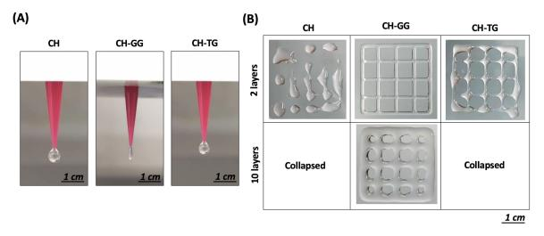
**Figure 3.1.** Printability of chitosan-guar gum and chitosan-tamarind gum biomaterial inks. (A) Initial screening of ink formulations through the extrusion of a small droplet and (b) printing of 2 and 10 layers in order to assess the successful layer stacking or the merging between layers.
