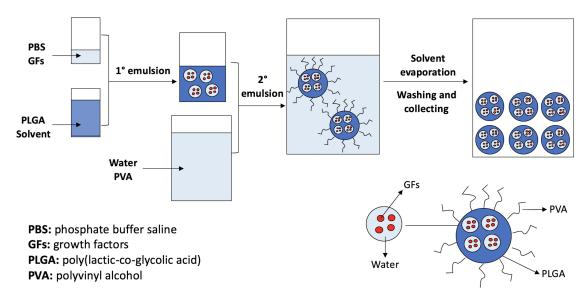
**Figure 5.3.** Preparation of PLGA microparticles by the double emulsion solvent evaporation method. Adapted with permission [266].
