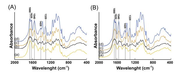
Figure A1. FTIR spectra of raw material (a), demineralized (b), deproteinized (c) and decolorized (d) samples extracted in (A) 2019 and (B) 2020.
