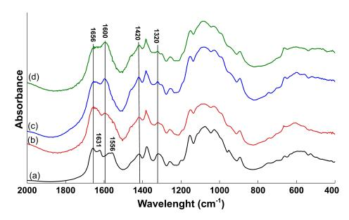
Figure 2.5. FTIR spectra of: (a) extracted chitosan, (b) CS-80, (c) CS-90 and (d) CS-95.
