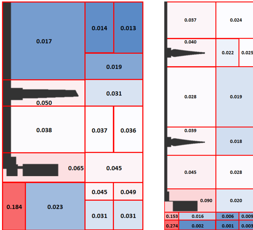
Figure 4.16: Representation of \langle k_1 a \rangle in each compartment for the laboratory- (left) and pilot-scale (right) tanks.
