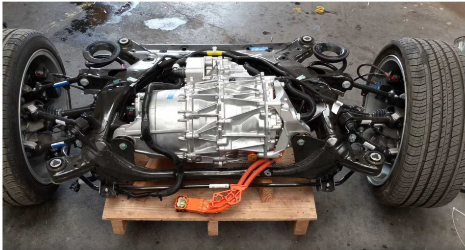
Figure 1.3 Tesla Model 3 drive unit [photo courtesy of CHARGED Electric Vehicles Magazine https://insideevs.com ] [5] [6].
